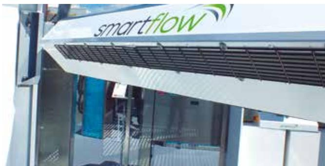
In addition to the full dryer (sides + top scanner), FLEX5 can incorporate the new Smartflow horizontal dryer patented by ISTOBAL to substantially reduce electricity use and noise levels.
